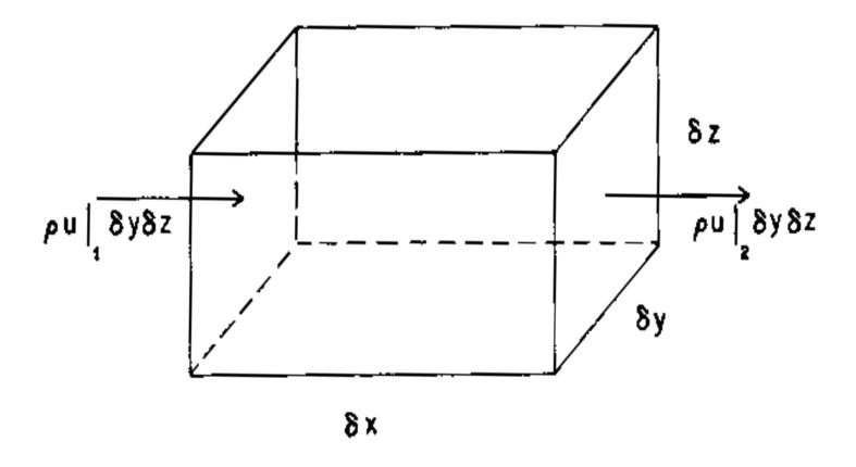
**Fig. 1.** A schematic of an infinitesimal box used to derive the conservation of mass relation
